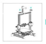
④ Install the screw rod fixing block from the top and tighten the screws.
